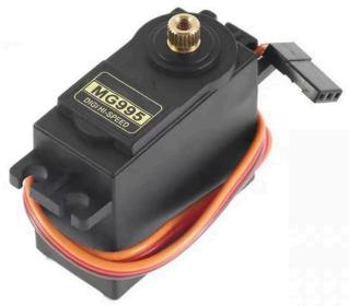
A black MG995 servo motor with a gold-colored horn and a black servo horn. It has three wires (red, yellow, and brown) and a black servo horn. The label on the motor reads "MG995". |
